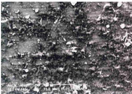
Fig. 3. SEM micrograph of the front surface of Cu substrate with 3 hours deposition.
