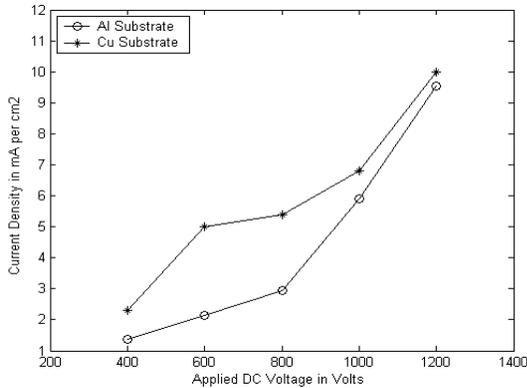
Fig. 2. Comparative plots of current density versus applied voltage for Cu and Al substrates.
