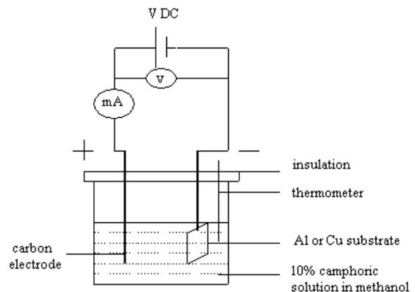
Fig. 1. Experimental set up of DLC film deposition on Cu and Al substrates
