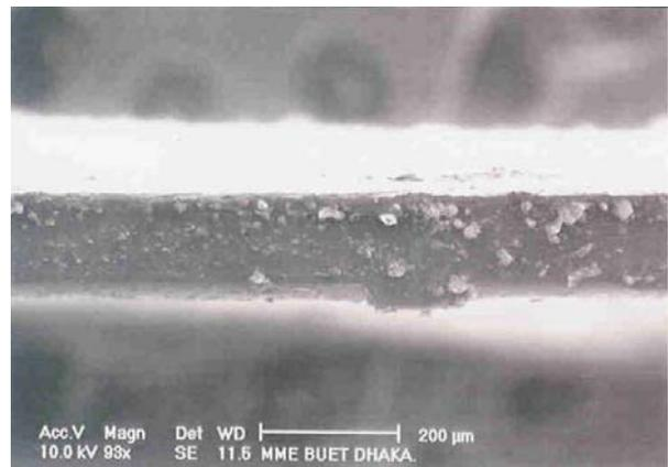
Fig. 6. SEM micrograph of the cross section of Cu substrate with 10 hours deposition.
