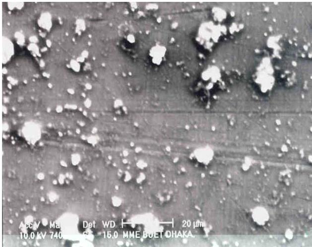
Fig. 8. SEM micrograph of the front surface of Al substrate with 10 hours deposition.
