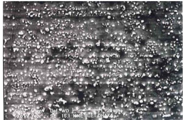
Fig. 5. SEM micrograph of the front surface of Cu substrate with 10 hours deposition.
