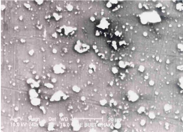
Fig. 7. SEM micrograph of the front surface of Al substrate with 4 hours deposition.
