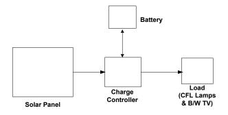
Fig. 1. Block diagram of a solar home system.
