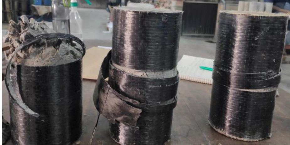
Figure 7: Failure pattern of cylinders wrapped in three layers.
