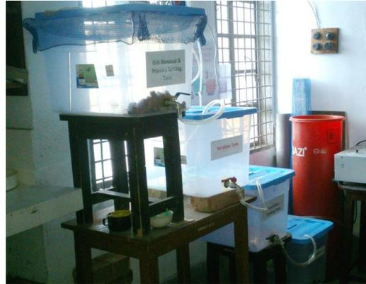
Figure 4: Laboratory Setup of Activated Sludge Treatment Unit.
