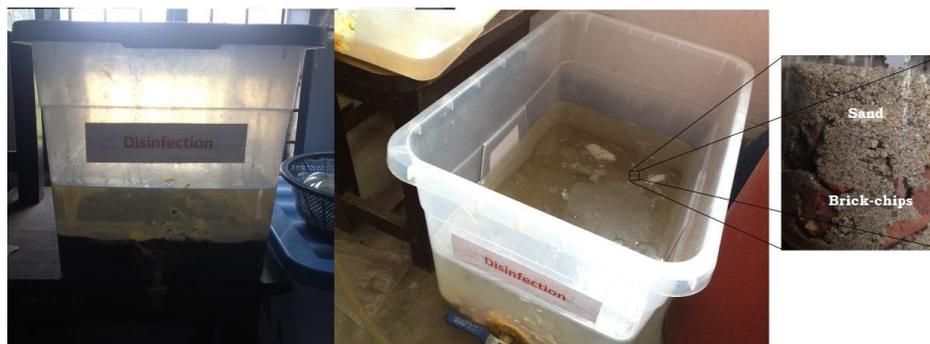
Figure 6: The Developed Upgraded Duel-Media Filtration Unit.
