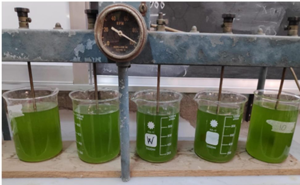
Figure 6: Jar test of microalgae coagulation and flocculation process.
