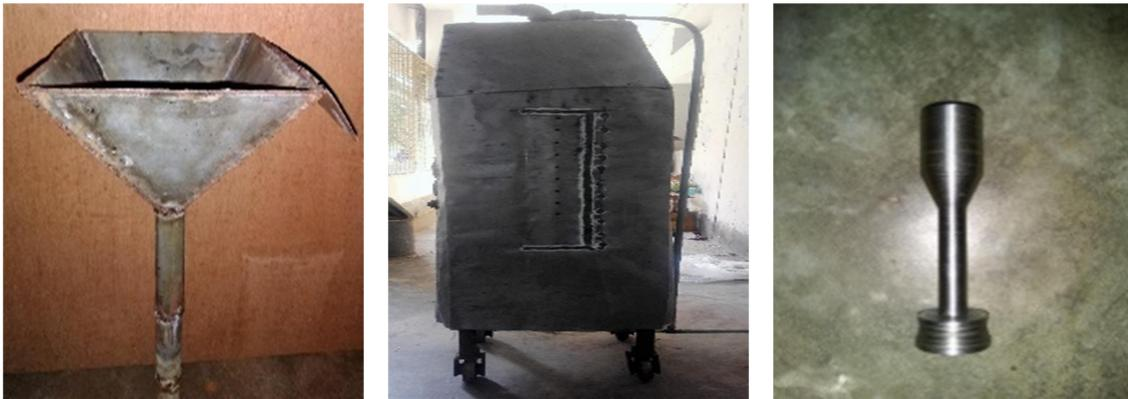
Figure 2: Different components of the setup (Left- Coal hopper, Middle- Furnace, Right- Burner).
