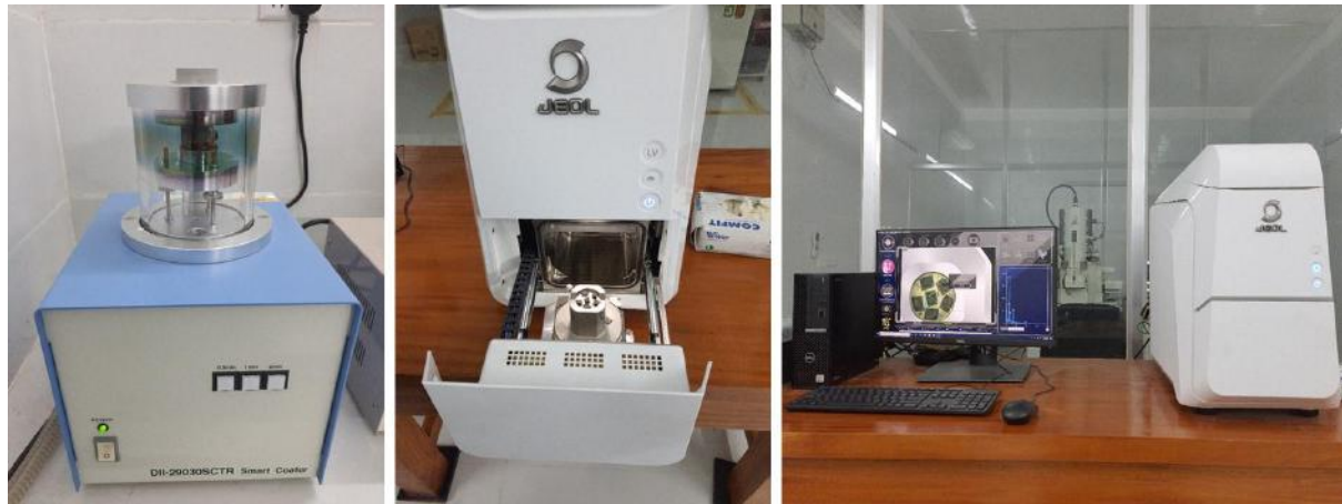
Figure 2: (a) Gold plating upon the sample, (b) Sample placement on JEOL-JCM-7000 NeoScope™ Benchtop SEM (c) Microstructure analysis through JEOL-JCM-7000 NeoScope™ Benchtop SEM
