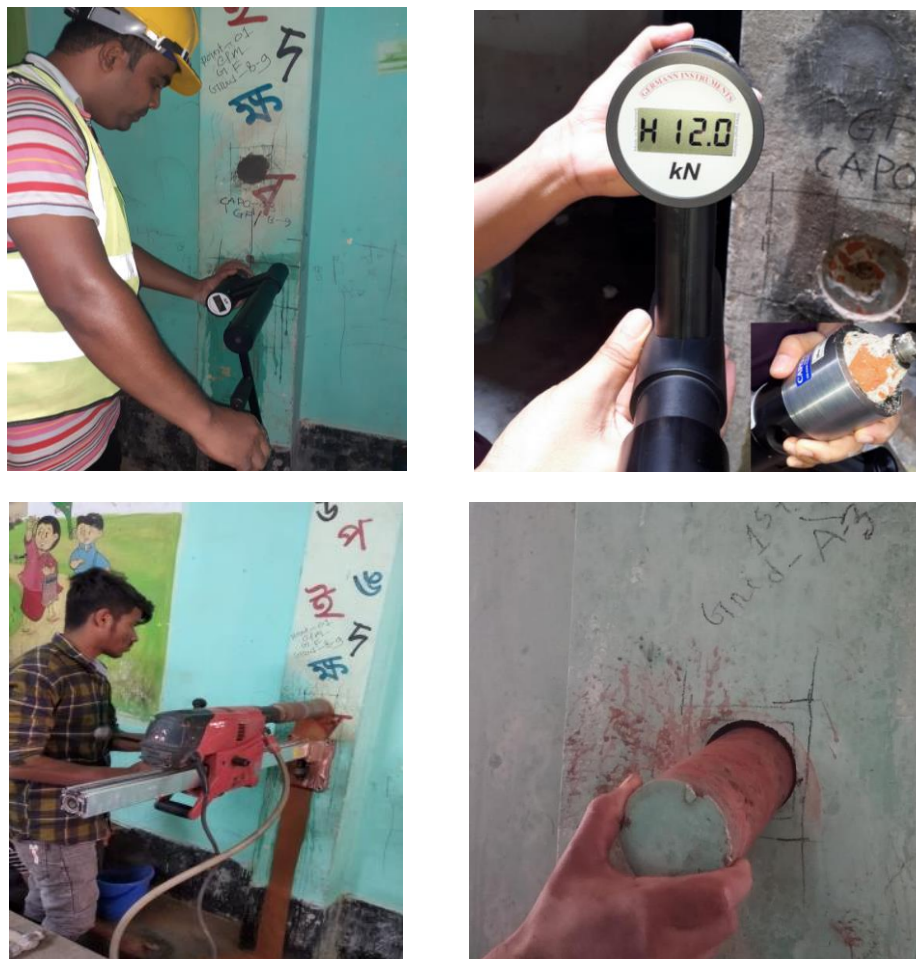
Figure 5: The CAPO-TEST (top row images) and core collection (Bottom row images) from a column
