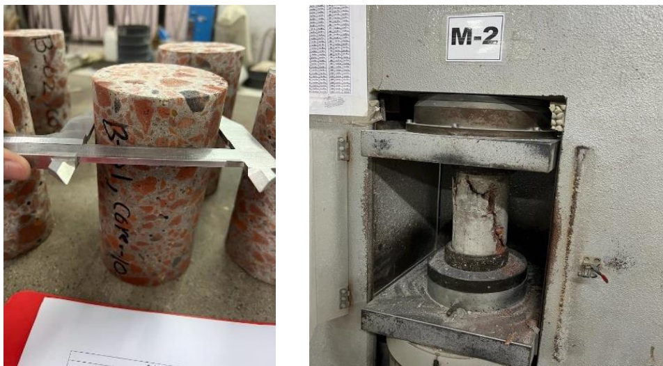
Figure 6: (a) Measure the core sample and (b) Testing of Cores
