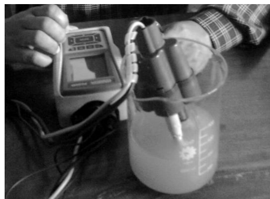
Fig 2: Testing of wastewater sample by Water Quality Monitor
