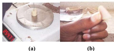
**Plate 1.** Gel forming test; (a) puncture test; (b) folding test
