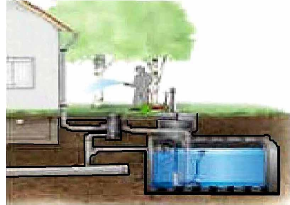
Fig. 2. Rainwater harvesting system at rural area in Bangladesh
