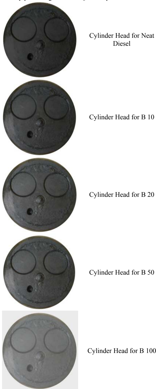
Figure 8: Cylinder head for Diesel engine by using neat Diesel, B10, B20, B50 and B100.
