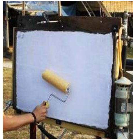
Figure 3. Wet handmade cotton paper sheet being applied to the drier surface with a roller.
