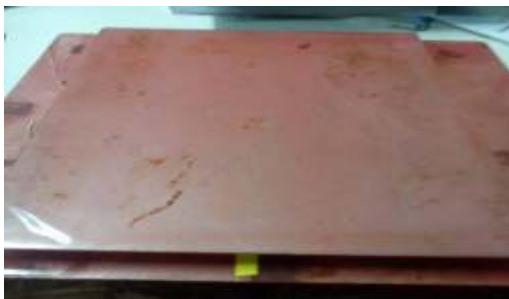
Figure 4. Clamping of layers before curing.
