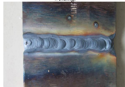
Figure 4. Broad view of heat affected zone developed in joint.
