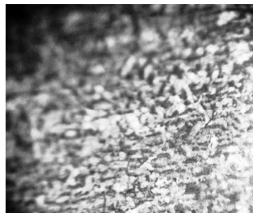
Figure 7. Microstructure of weldment for electrode wire diameter 0.8 mm, wire feed rate 4600 mm/min and current 240 amps.
