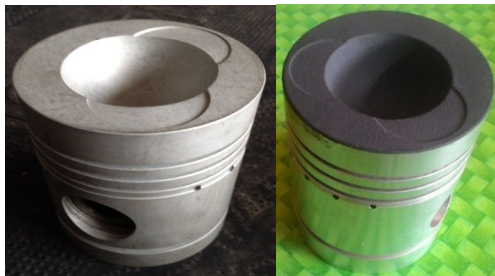
Figure 3. Pistons before and after coating with TiO 2 powder
