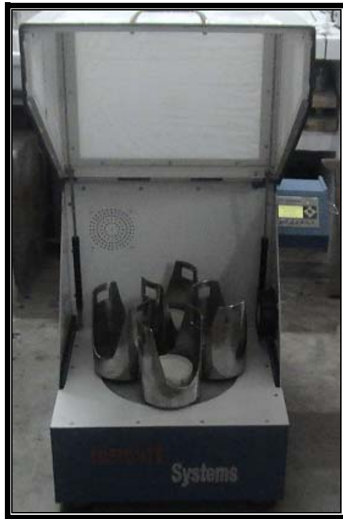
Figure 1(a). Planetary High Energy Ball Mill
