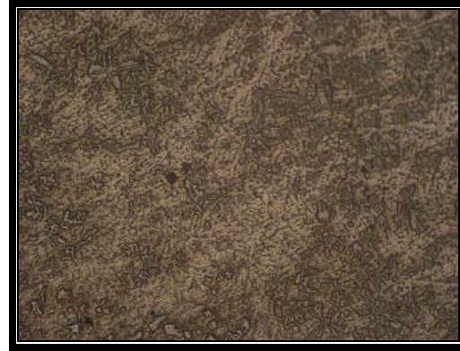
Figure 6(c). Optical microstructure of A356 matrix reinforced with 0.5Wt% of micro SiC particles (125µm) at 200x magnification.
