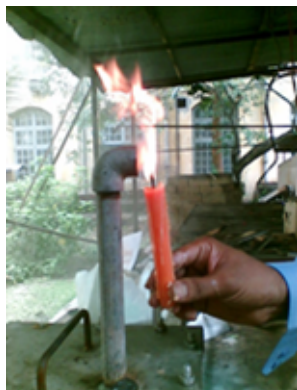
Figure 5: The producer gas is being ignited
