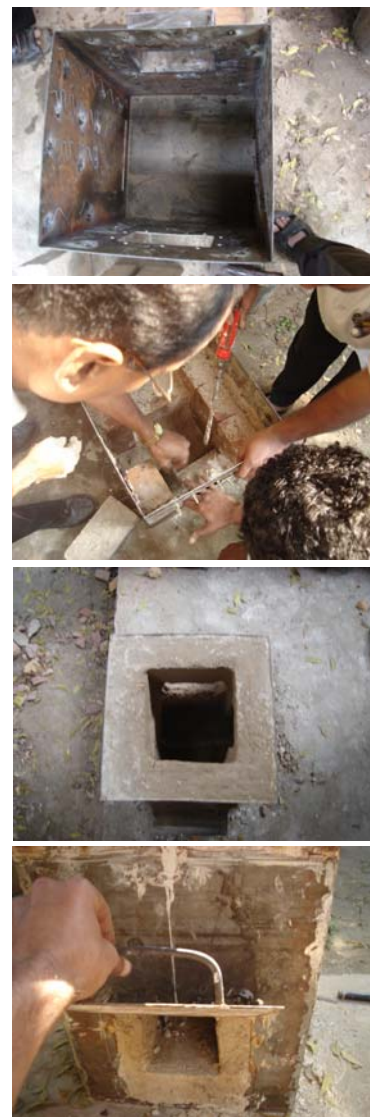
Figure 3: Photograph of the Reaction Chamber. Top: without bricks; Upper middle: with bricks; Lower middle: plastered with refractory cement; Bottom: ash removal door.
