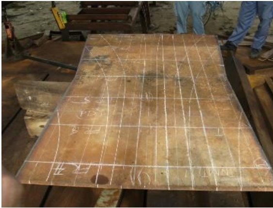
(a) Mark the heating line on the initial planar plate
