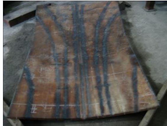
(b) Shape of the curved K1 plate after forming
