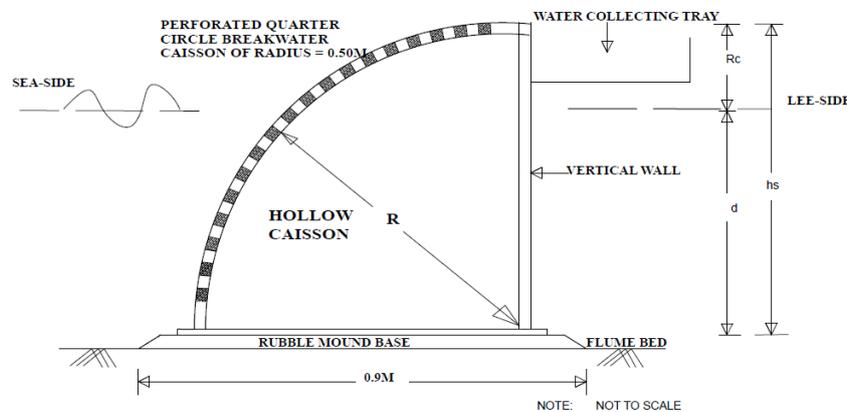
Fig. 3b: Typical cross-section of a seaside perforated QBW
