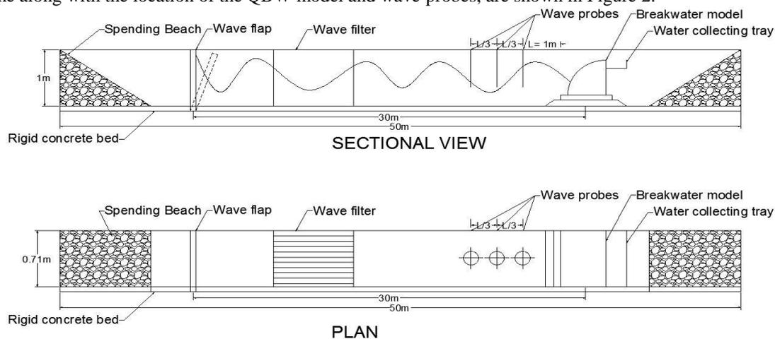
Fig. 2: Wave flume arrangement (Not to scale)
