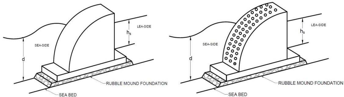
Fig. 1: Isometric view of non-perforated and perforated QBW
