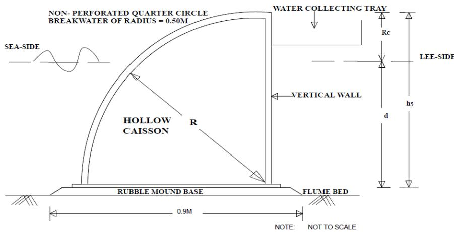
Fig. 3a: Typical cross-section of non-perforated QBW
