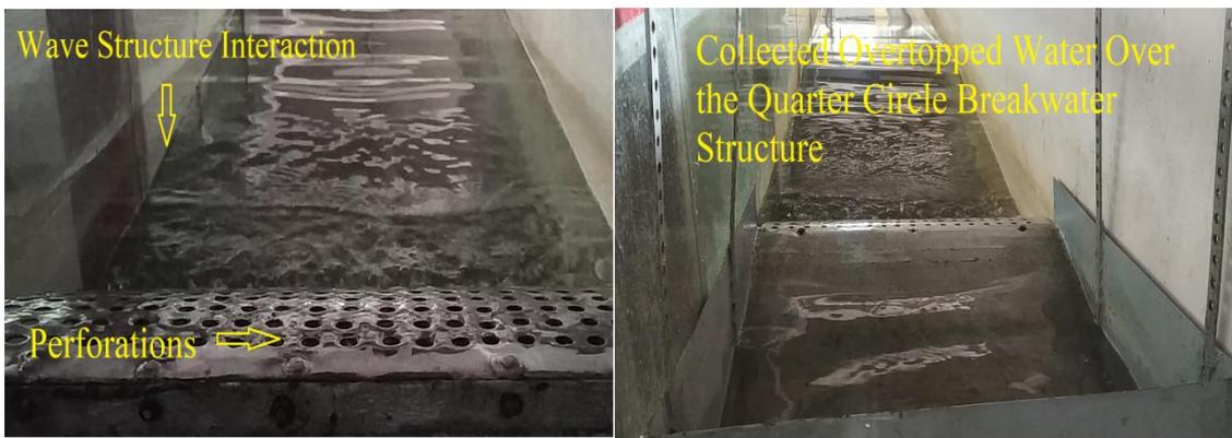
Fig. 4b: A typical front and rear view of water collected in a tray
