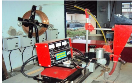
Fig. 4: SAW machine (MODEL PS-1200(F)) setup.
