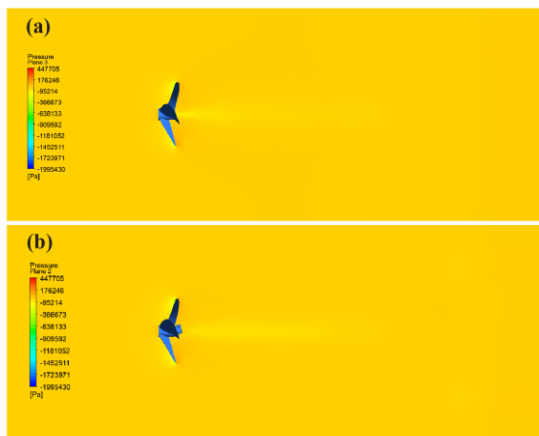
Fig. 28: Pressure contour at J = 0.415 (a) Baseline Propeller without PBCF (b) Propeller with modification PBCF
