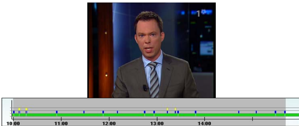
Fig. 9 TV channel measurement graph from Agama. Green=OK, Blue=minor distortion, Yellow=major distortion, Red=Packet loss.
