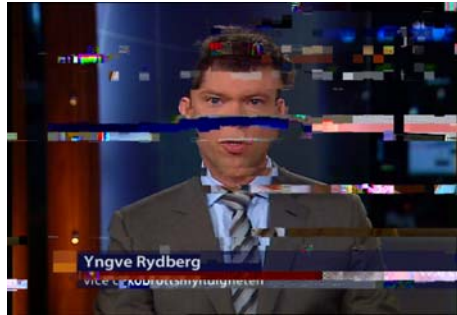
Fig. 1. Effects of packet loss in IPTV service.
