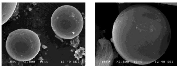
Fig. 4. SEM photograph of nicorandil microsponge formulation (Batch F6).
