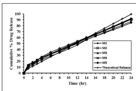
Fig. 5. The in vitro drug release profile of nicorandil from M1-M5 formulations.
