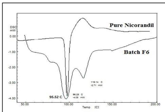
Fig. 3. DSC thermograms of pure nicorandil and microsponge formulations (Batch F6).
