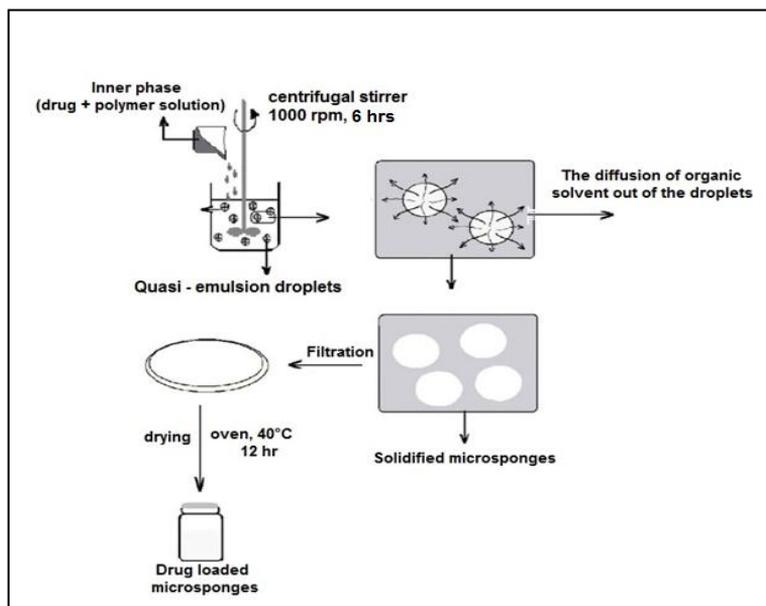
Fig. 1. Preparation of microsponges by quasi-emulsion solvent diffusion method.
