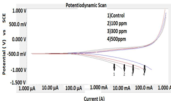
Fig. 5. Potentiodynamic polarization curves for mild steel without and with different concentrations of MIZ in *Barr's* medium inoculated with SRB.
