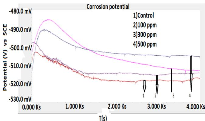
Fig. 3. Open circuit potential of mild steel without and with different concentrations of 2-methylimidazole (MIZ) in *Barr's* medium inoculated with SRB.
