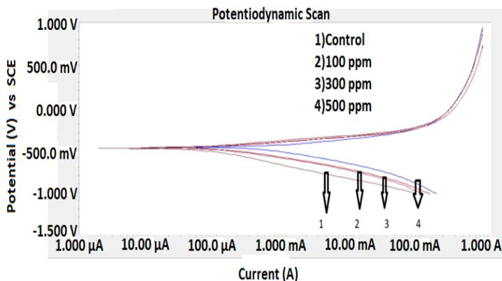
Fig. 4. Potentiodynamic polarization curves for mild steel without and with different concentrations of MNZ in *Barr's* medium inoculated with SRB.
