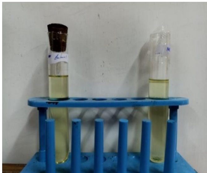
Fig. 1. Stability test: Sample 1 (D70WCO10WCCO15Bu5) and Sample 2 (D70WCO10WCCO15Me5).
