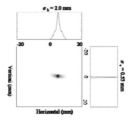
Fig. 2. Simulated beam profile in FIR region ( $\sim 100 \text{ cm}^{-1}$ ) at first focal point. The beam size is smaller than that of the electron beam. Note that the beam profile is slightly shifted from the origin in horizontal. This might be due to a large horizontal acceptance angle of 264 mrad.
