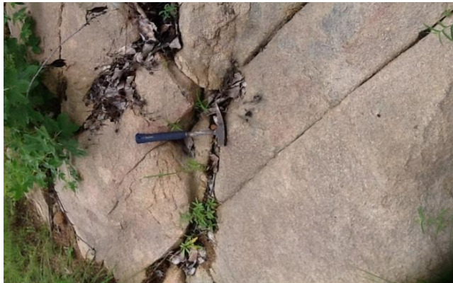
Fig. 6. Shear Fractures in granite rock around Shintaku.
