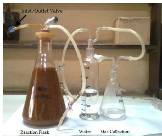
Fig. 1. Working model of bioreactor for biogas production.
