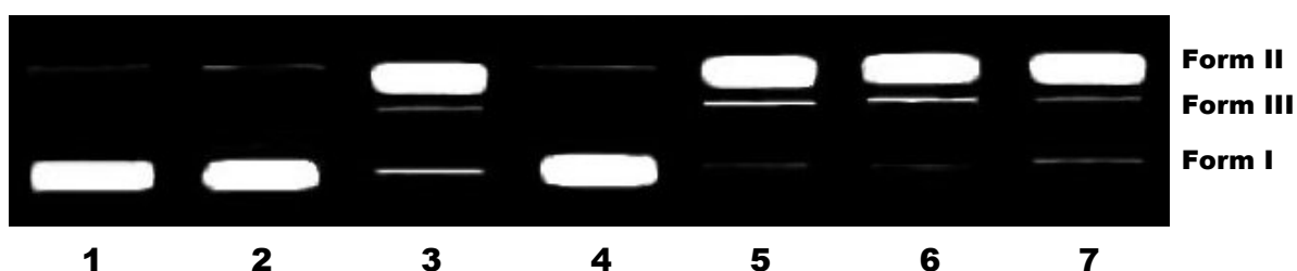
Fig. S36. Gel electrophoresis diagram showing the cleavage of 20 \mu\text{M} SC pUC19 DNA by 3 (30 \mu\text{M} ) in a 2% DMF/5 mM Tris-HCl/50 mM NaCl buffer at pH 7.1 and 37 ^{\circ}\text{C} in the presence of \text{H}_2\text{O}_2 (200 \mu\text{M} ). with an incubation time of 2 h: lane 1, DNA control; lane 2, DNA+ 3 ; lane 3, DNA+ 3 + \text{H}_2\text{O}_2 ; lane 4, DNA+ 3 + \text{H}_2\text{O}_2 +DMSO (20 \mu\text{M} ); lane 5, DNA+ 3 + \text{H}_2\text{O}_2 +SOD (0.5 units); lane 6, DNA+ 3 + \text{H}_2\text{O}_2 + \text{NaN}_3 (100 \mu\text{M} ); lane 7, DNA+ 3 + \text{H}_2\text{O}_2 +Catalase (6 unit).
