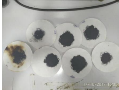
Fig. 2. Circular shaped dispersed CNT residue CNT on filter paper.
