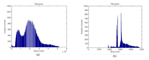
Fig. 4. Histogram of CT image (a) after histogram equalization, and (b) after enhancement using local statistics.
