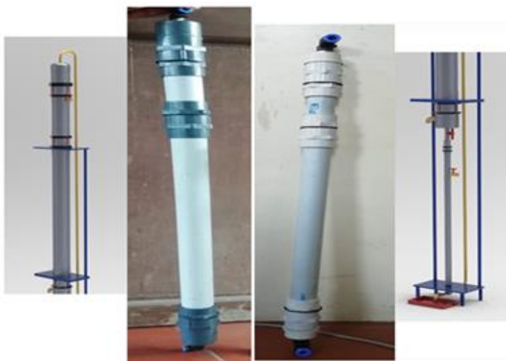
Fig. 7. Fabricated VMFB with the lower anaerobic and upper aerobic zone.
