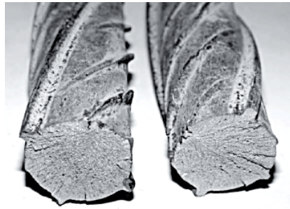
Fig. 7. Brittle type failure during bending test of a conventional high strength reinforcing steel bar.
