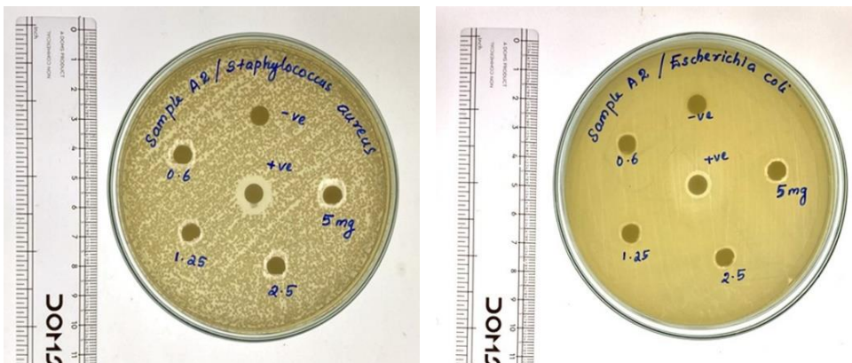
Fig. 11. Anti-bacterial activity of TeO 2 -SeO 2 nanocomposite coating on Ti substrate with highest inhibitory action against Staphylococcus aureus and Escherichia coli , respectively.
