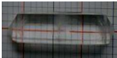
Fig. 9. Photograph of the as grown crystal of 0.5 mol% EDTA added KDP.
