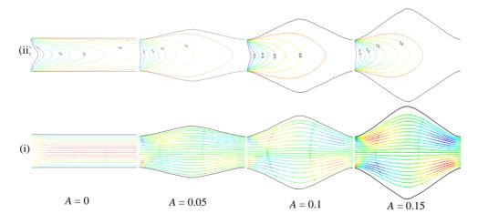
Fig. 6. Effect of A on (i) streamlines and (ii) isotherms at Pr = 6.2.
