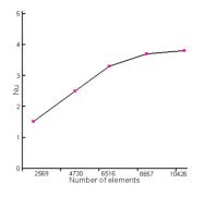
Fig. 3. Grid independency study for Da = 100, Re = 100, Pr = 6.2, A = 0.1 and  $\phi = 5\%$ .
