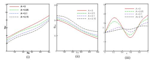
Fig. 7. (i) Rate of heat transfer, (ii) mean temperature and (iii) mid-height U-velocity for different A.
