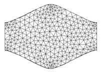
Fig. 2. Mesh generation of the channel.
