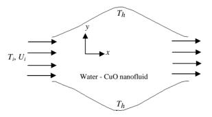
Fig. 1. Depiction of the geometry and the operation of the channel.
