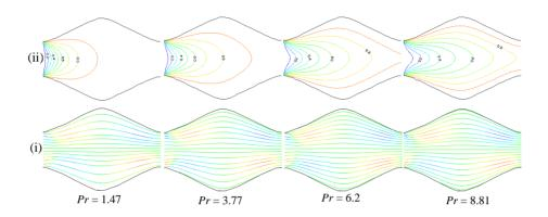
Fig. 4. Effect of Pr on (i) streamlines and (ii) isotherms at A = 0.1.
