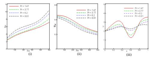
Fig. 5. (i) rate of heat transfer, (ii) mean temperature and (iii) mid-height U-velocity for different Pr.
