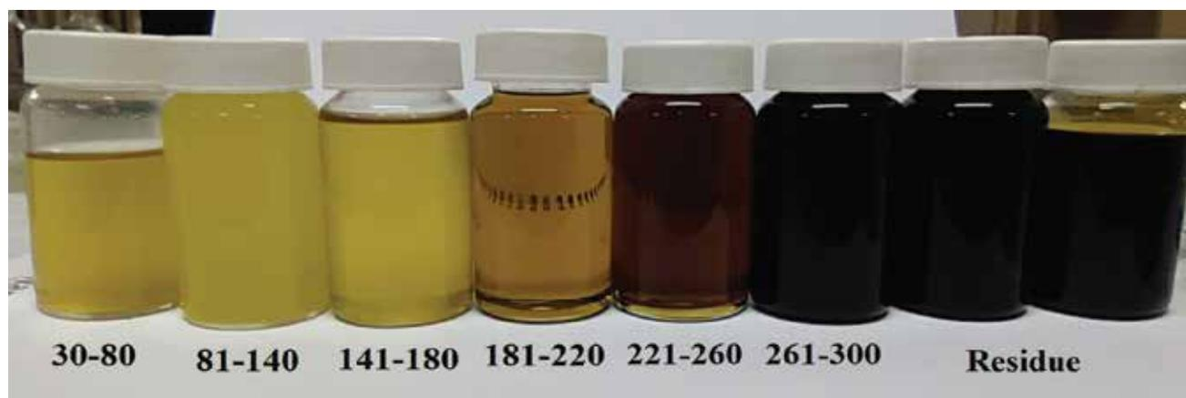
Fig. 5. Various fractions of liquid products distilled out from TPO
