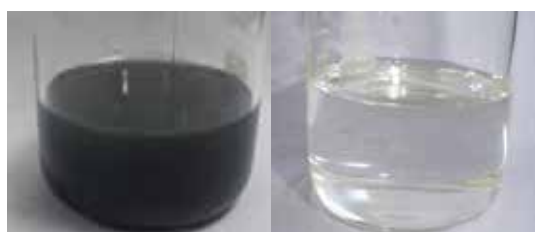
Fig. 2. (a) wPVC based solvent cement and (b) Virgin PVC based solvent cement.
