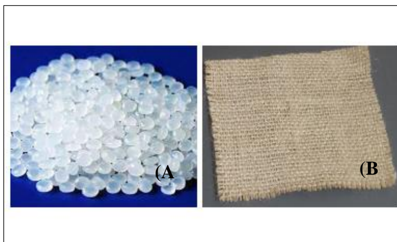
Figure 1. Digital images of polypropylene granules (A) and JF (B).
