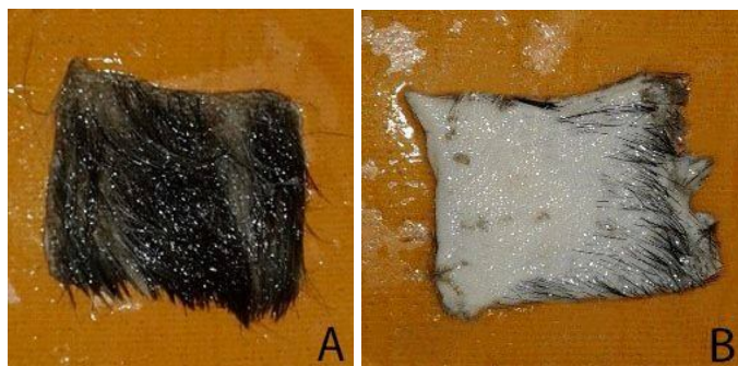
Fig. 6. Dehairing activity of protease at room temperature after 24h in water on goat skin (A) control-goat skin incubated at room temperature without protease, (B) Dehaired goat skin with protease from R82
