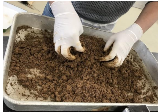
Figure 2. Mixing water manually with air-dried soil to reach the expected water content
