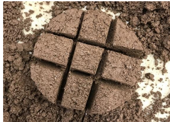
Figure 3. Sample collection from the central part of a layer in a specimen
