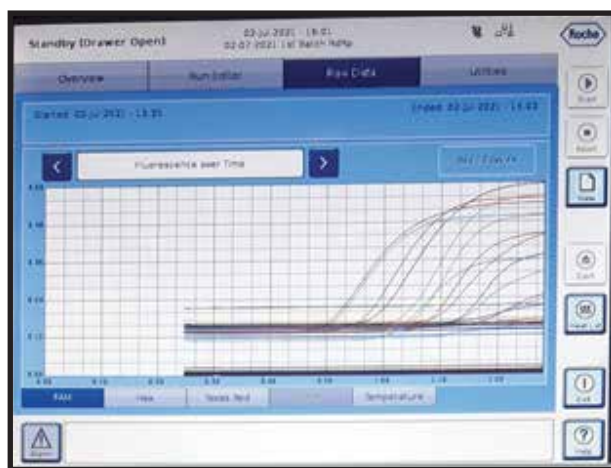
Fig 1: Fluorescence amplification signal curve over time in Realtime thermal cycler
