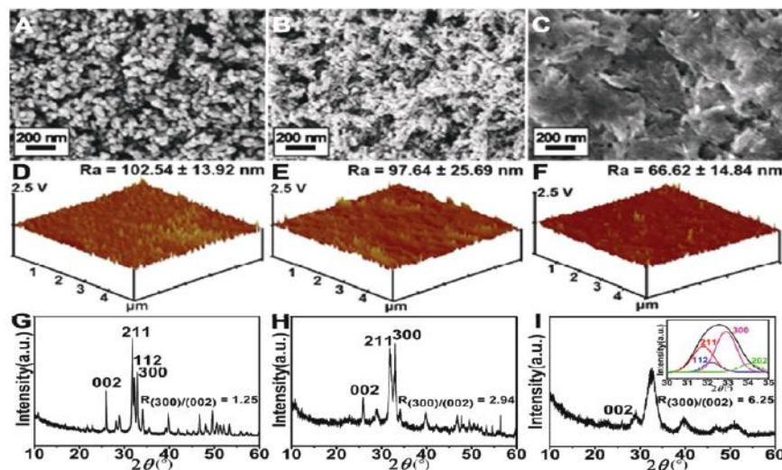
**Figure 03: Characteristics of different HAP films. The SEM images show different features**
