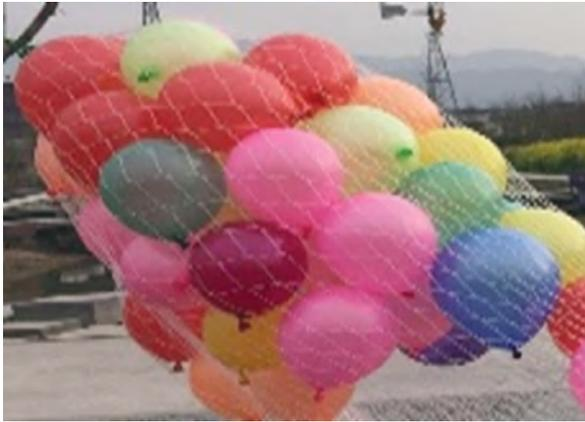
**Figure 05: Balloon-in-nylon-nets droplet catcher 30**
