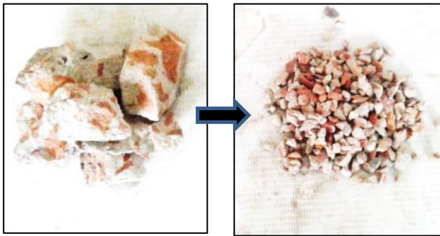
Figure 1: Demolished brick concrete block and recycled brick aggregates
