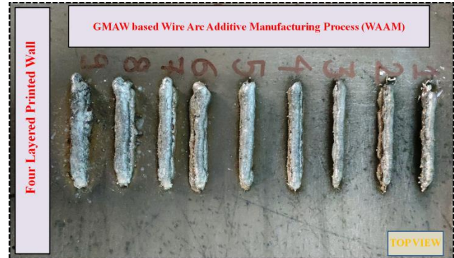
Figure 2: Fabricated WAAM specimens with different Heat Inputs
