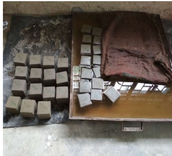
Figure 3. Curing of the cubes
