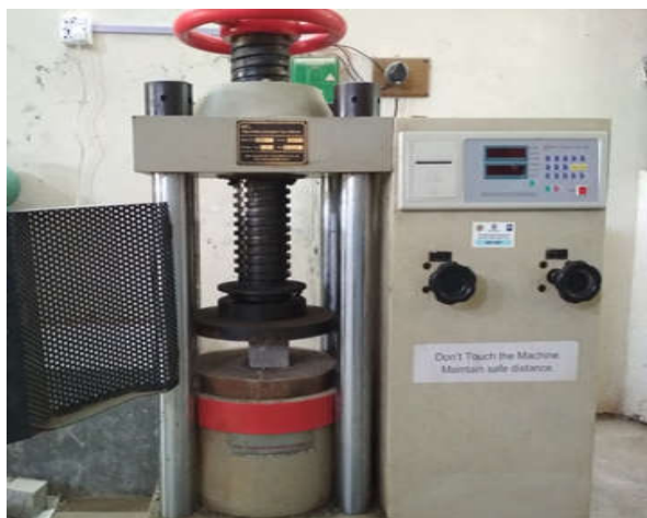
Figure 4. Compressive strength test
