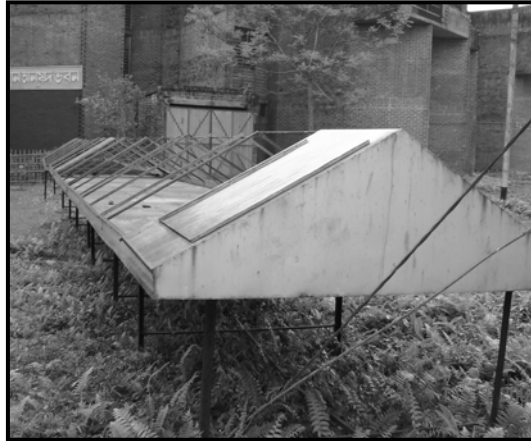
Plate No. 3. Solar tunnel dryer used for drying
