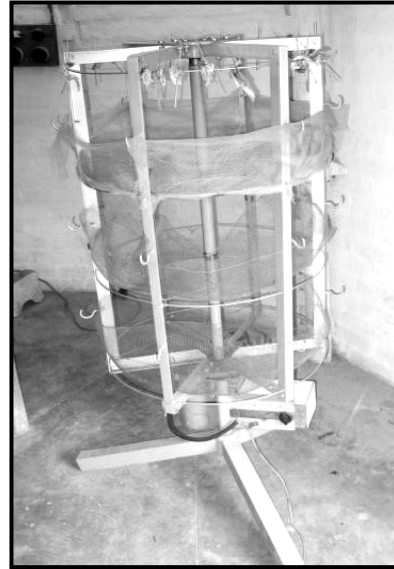
Plate No. 2. Rotating dryer with fish
